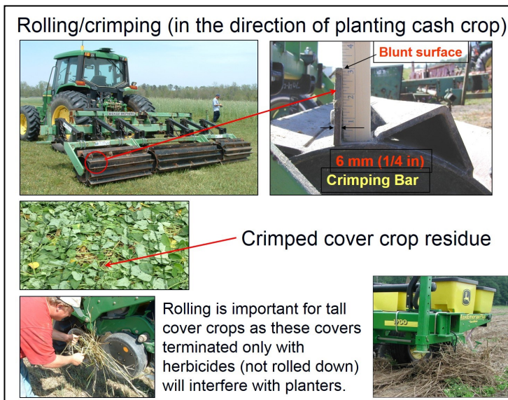
Fig. 1. Principle of rolling/crimping (in the direction of planting cash crop). All photos T. Kornecki
