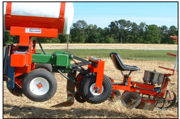
Fig. 6. Modified RJ transplanter by adding sub-frame with a subsoiler.
