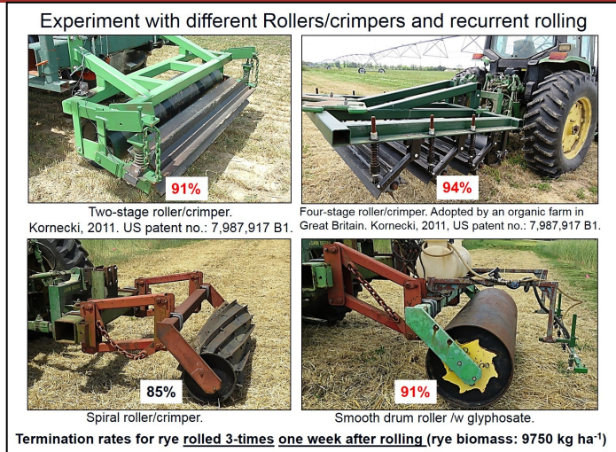
Fig. 3. Two-stage roller/crimper; four stage roller/crimper; curved roller/crimper and smooth drum roller with herbicide sprayer.
