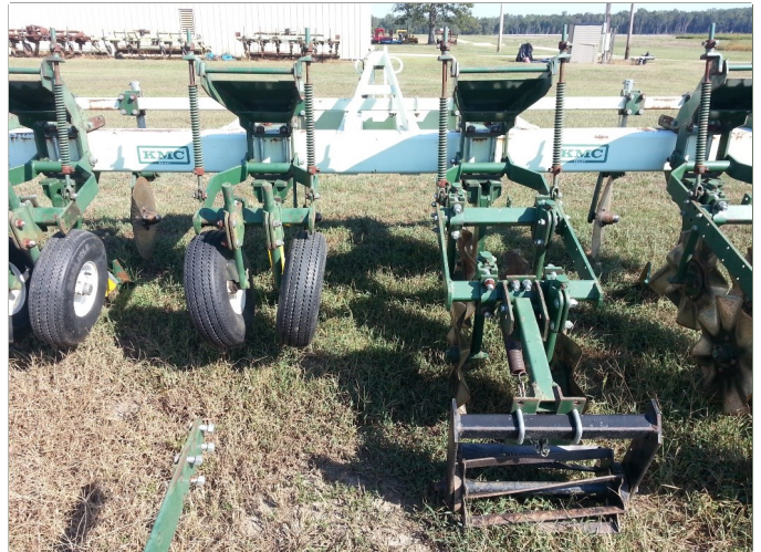
Fig. 6. An example of two different strip tillage configurations designed to create a narrow zone of surface soil disturbance (left) compared to a wider zone of surface soil disturbance (right). Photo courtesy of USDA-ARS, NSDL
