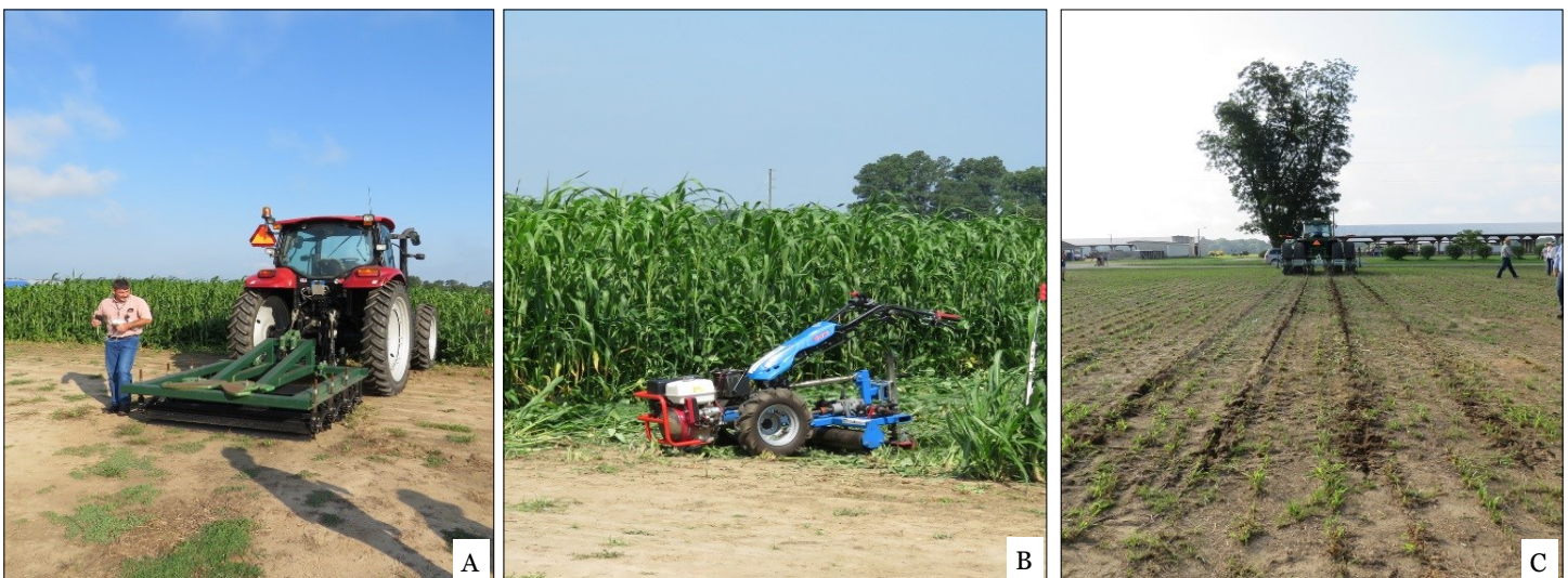
Fig. 4. Staff from NSDL demonstrated termination of a high-residue cover crop using a four-stage roller/crimper (A) and a powered roller/crimper for walk-behind tractors (B), as well as a strip tillage implement with different strip tillage attachments (C). Photos courtesy of USDA-ARS, NSDL
