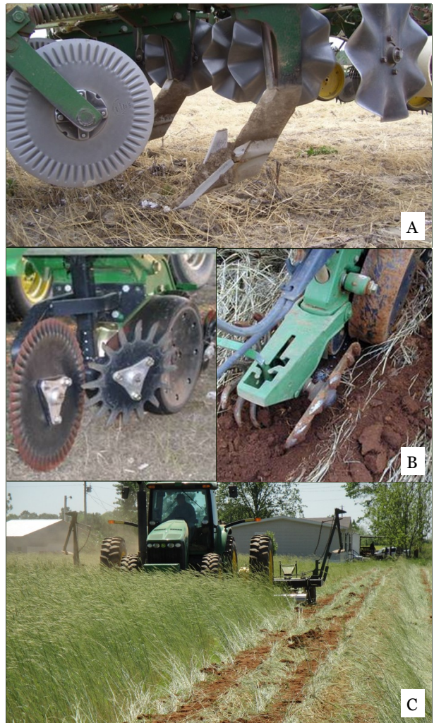
Fig. 4. Example of tillage shank with coulter (A), row cleaners and closing wheels (B), and a combined operation (C) for residue management. Photo courtesy of USDA-ARS, NSDL
