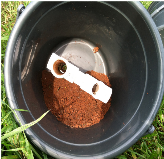
Figure 12. Both units were used to sample an equivalent number of soil cores. This design not only showed no torque force on the pipe, but also showed little sign of soil buildup inside the pipe.
