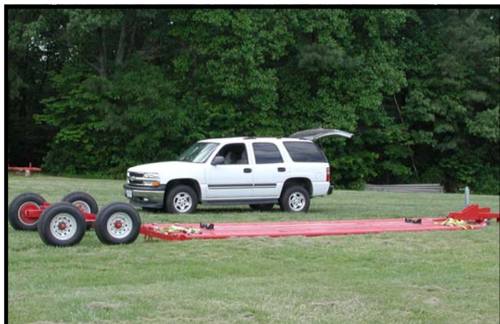
Our special trailers can lay flat on the ground if needed, so rollers can be loaded and unloaded without lifting.
