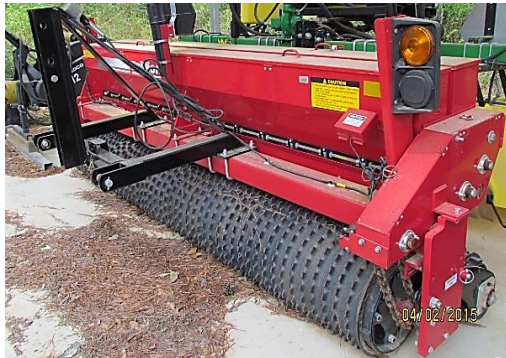
Brillion seeder for conventional prepared seedbeds.
