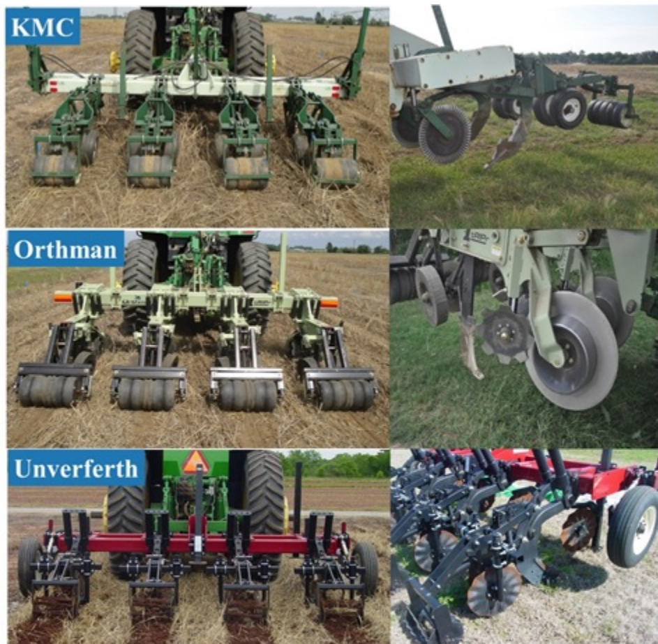
Figure 1. Strip tillage implement, corresponding shanks, and attachments used in the peanut study in Headland, AL and Tifton, GA. Tillage depths were ~13 to 14 inches for implements.
