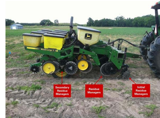
Figure 2. No-till planter with an added front toolbar to aid with planting into heavy residue cover crop mulches.
