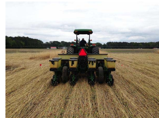
Figure 4. Planting cotton into a roll-killed cereal rye and crimson clover cover crop mulch with the initial residue managers floated at planting.
