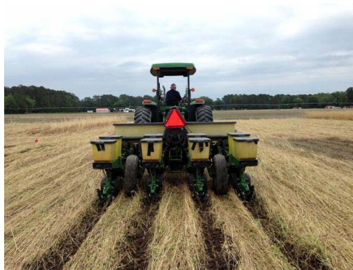
Figure 3. Planting cotton into a roll-killed cereal rye and crimson clover cover crop mulch with the initial residue managers engaged at planting.
