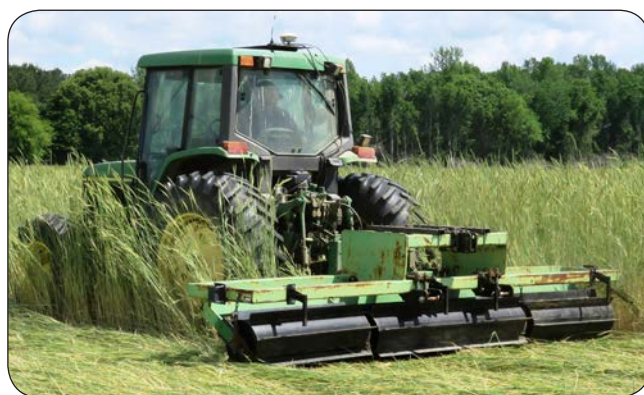
Straight crimping bar roller/crimper
