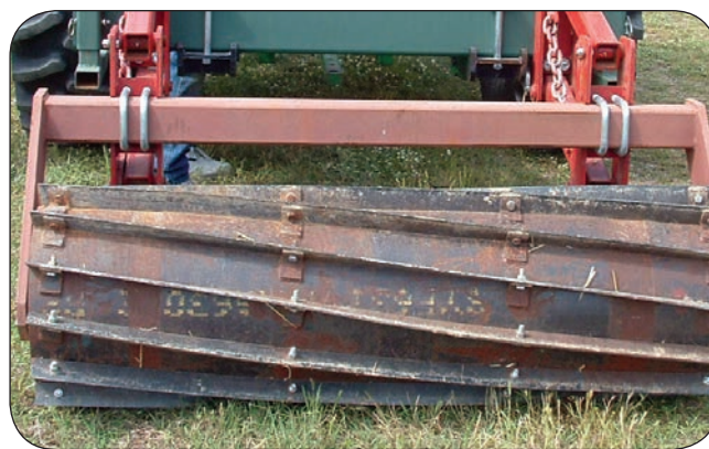
Curved crimping bar roller/crimper
