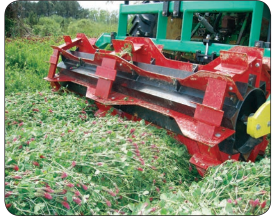
Rotary roller/crimper for elevated bed culture
