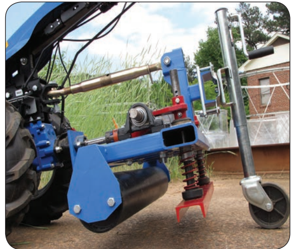
Powered roller/crimper for walk-behind tractors
