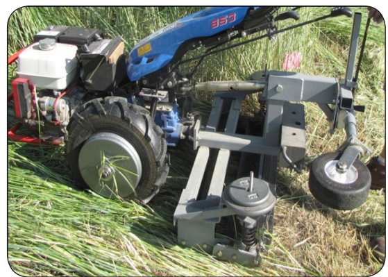
Two-stage roller/crimper for walk-behind tractors
