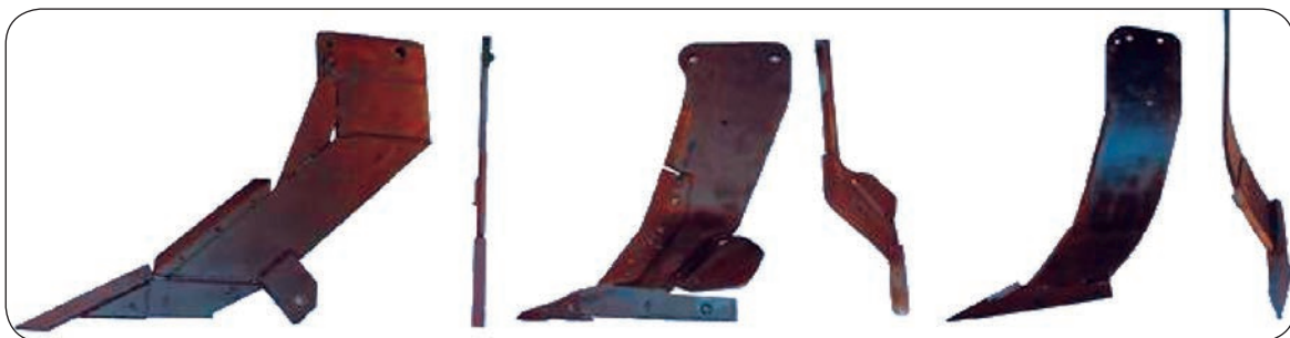
Side and front view of an in-row subsoiler (left) and two bent-leg subsoilers.
