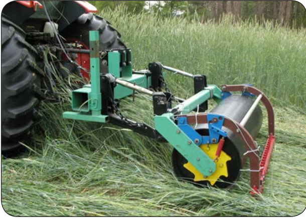
Smooth roller with oscillating crimping bar assembly
