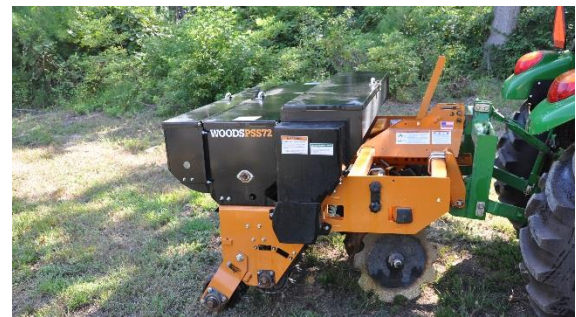
An all in one planter with 3 seed box configuration. The front disks prep the seed bed. Seed falls to the ground behind the disks, and the rear cultipackers seal it. Note the paint missing on the fluted disk indicating the shallow soil disturbance of this planter. The angle of attack on the disks is adjustable via the orange handle to increase or decrease the soil disturbance.
