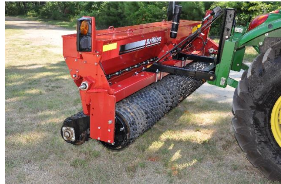
A typical drop seeder with two sets of cultipackers. Seed falls from the seed box between these rolling cultipackers during planting. These are typically used with small seed.
