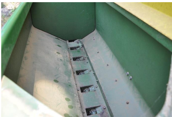
The inside of a standard seed box showing the gravity fed mechanism that delivers seed to drop tubes. Seed is metered out via rollers with gear like teeth in the openings that control the rate seed flows to the drop tubes.
