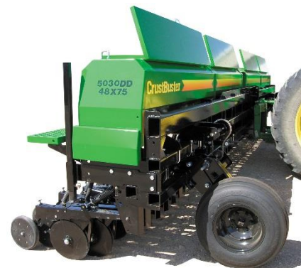
A grain drill with a standard seed box, note the V openers and press wheels with no fluted coulters.
