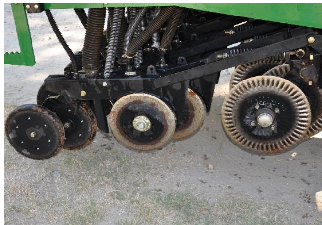
The front fluted coulter of a no-till drill slices an opening through hard sods for the “V” openers, seen middle, to open and deposit seed. The spring loaded press wheels then seal the opening.
