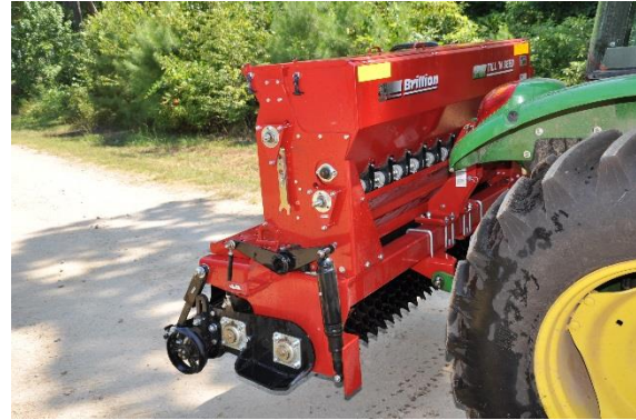
The Till 'n Seed model from Brillion is an all in one planter that creates a very shallow seed bed, less than an inch. The counter rotating sprockets can be seen in the photo under the planter
