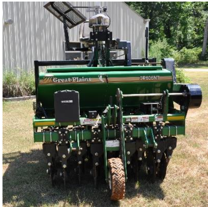
Front view of a no-till drill showing the rubber drive wheel, center. This planter has an optional research plot option attached to the top; not typical of standard drills used in conservation plantings.
