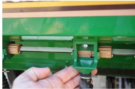
The smaller seed delivery mechanism of a legume seed box on a no-till drill. Large seed will jam the small gears that deliver seed to the drop tubes.
