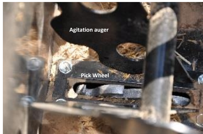
Close up view of the agitation auger and the pick wheel inside a native seed box. The gear like teeth on the pick wheel reaches into the seed box, grabs seed, and pull it down into the drop tubes at a steady rate rather than relying on gravity to feed the mechanism. The auger blades move seed back and forth to keep it constantly moving and prevents seed from bridging on itself.
