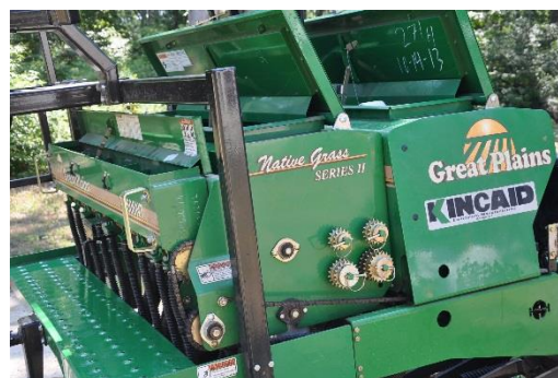
Side view of a no-till drill with a 3 seed box configuration for legumes, native grass, and standard seed. Note the size difference of the legume seed box, first box on left.
