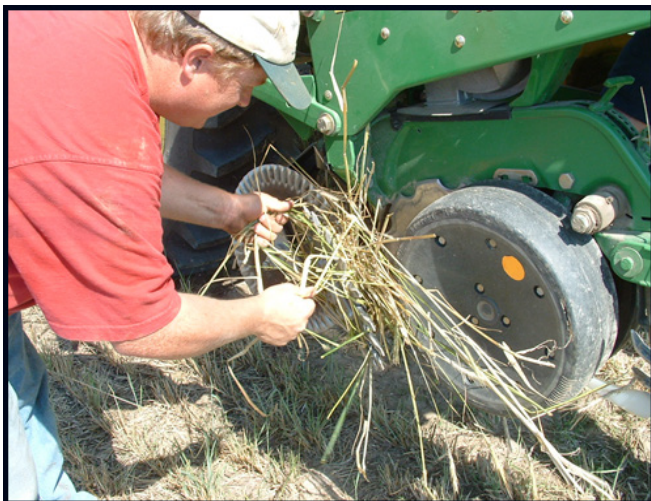
Figure 3. Removing residue that becomes entangled in equipment can waste considerable time leading to grower frustration with cover crops.
